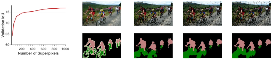
Fig. 6. Hierarchical Clustering Analysis. From left to right: Validation performance when using different super-pixel layouts, visualization of an image with ground truth segmentation, and the BI_6(2) - BI_7(6) result with 200, 600, and 1000 superpixels.
